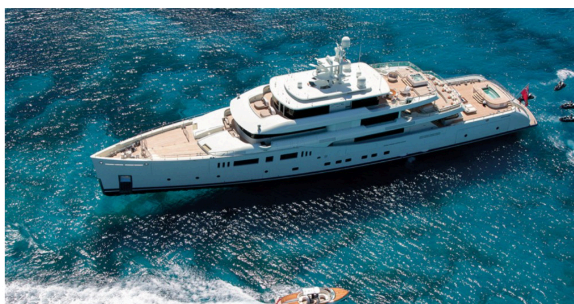
The 240-foot Nautilus has a more classic megayacht look than its sisterships, but shares the vertical bow and low-slung decks. Courtesy Philippe Briand
